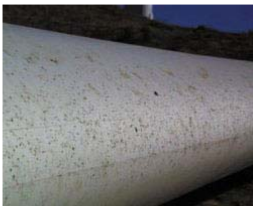
Insect bodies litter a wind-turbine blade's leading edge.
